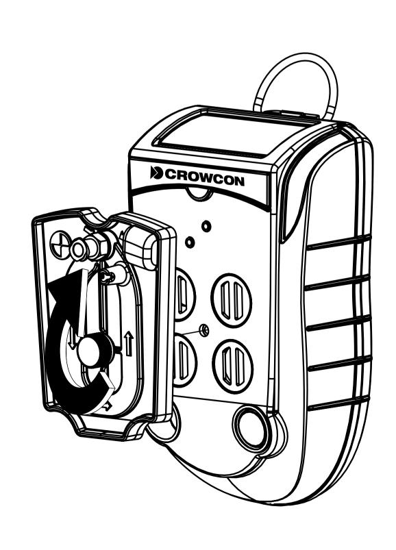
Figure 5: Fitting a flow plate
