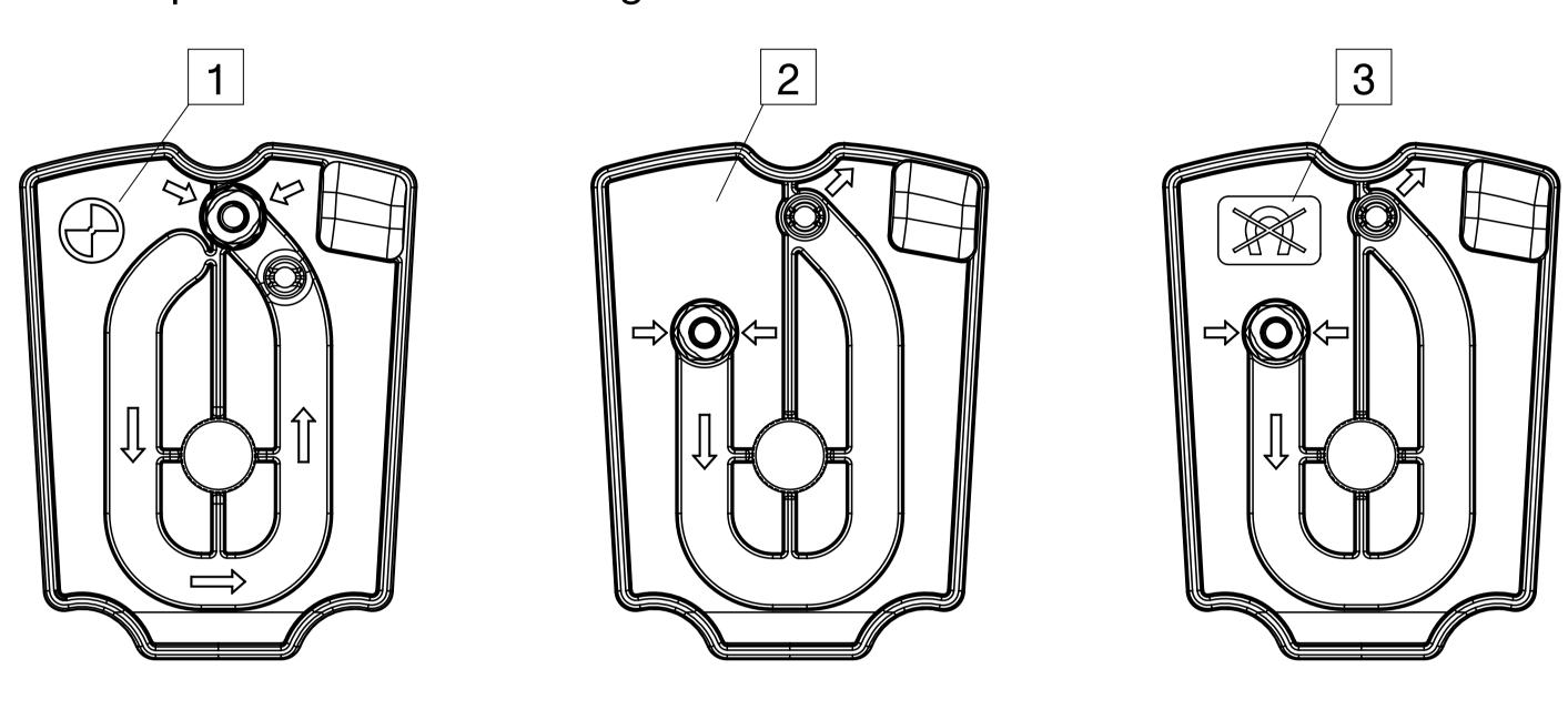
Figure 4: Pumped and non pumped flow plates
